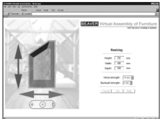
Figure 3. The closet's size can be altered either by typing the absolute values, or by directly dragging the closet's walls. The visual and tabular presentations are updated simultaneously. Any shelves or doors that have already been added to the closet are reshaped and repositioned to fit the new closet geometry.
