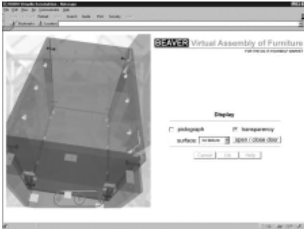
Figure 5. Fittings and hinges can be examined during the design phase if the model display type is set to transparency. In BEAVER, the user needs not care about which type of fitting he should use or where to place the fittings. BEAVER finds the optimal configuration of fittings for the specific closet designed.
