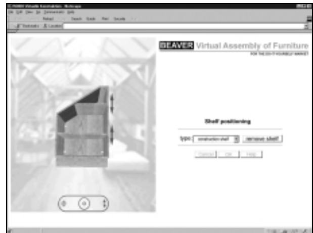
Figure 1. Virtual assembly with BEAVER. Shelves can be added, removed from, or shifted inside the 3D closet model. The program automatically calculates the required size and shape of the shelves, while they are moved to different positions.
