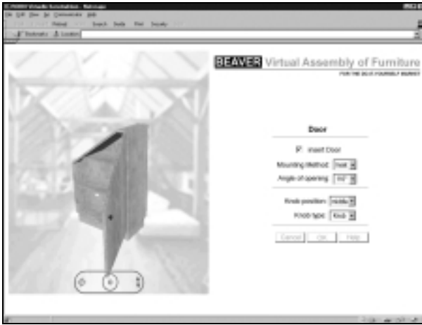
Figure 2. Virtual prototyping allows testing of the model's functions before its real assembly. With BEAVER, for example, the opening angle of the closet can be experienced.
