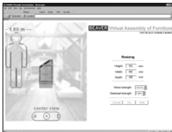
Figure 7. The navigation console is a part of the initial VRML world. In addition to the tabular presentation of the closet's size, a pictograph of a human figure can optionally be displayed in the virtual workroom, lending the user a visual impression of the closet's size.
